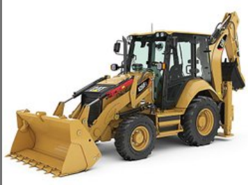
CAT 424B Backhoe Loader
