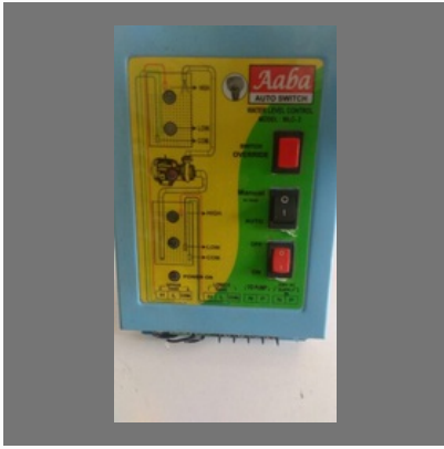
Water Level Controller
