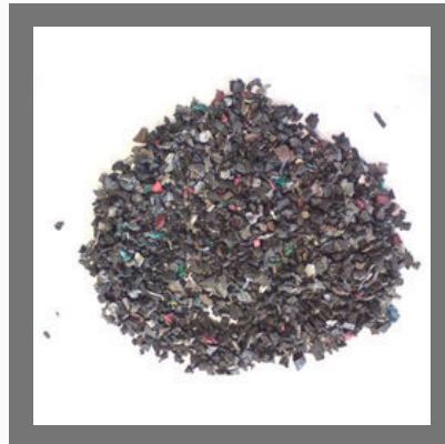
PVC Cable Scraps
