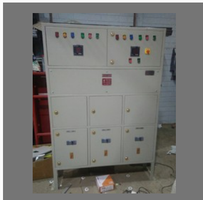
Genset AMF Panel
