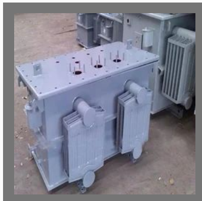
Distribution Transformer Body
