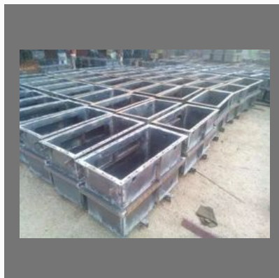
Transformer Fabricated Tank
