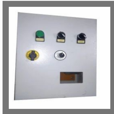
Single Phase AC Drive Panel
