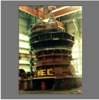
Primary Gyratory Crusher
