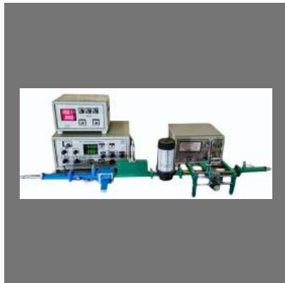
MICROWAVE TEST BENCH SET UP (KLYSTRON POWER SUPPLY) HIQ 6100
