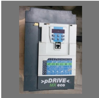
P Drive, MX Eco-drive( Frequency Inverter)
