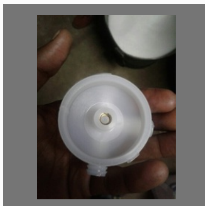
Cooler Pump Distributor
