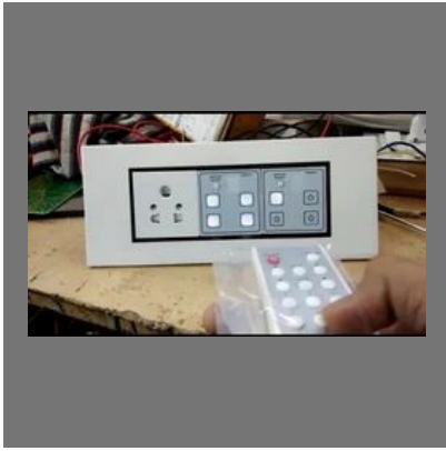
Remote Control Switches
