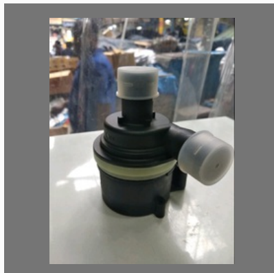
Additional Water Pump
