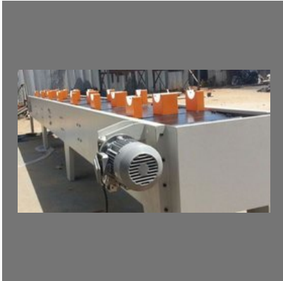
Assembling Chain Conveyor
