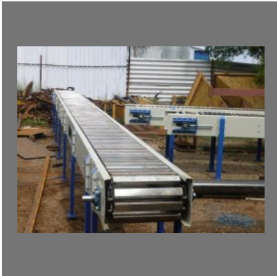
SS Chain Conveyor
