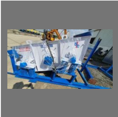
20x06" Stone Crusher Vibrating Screen
