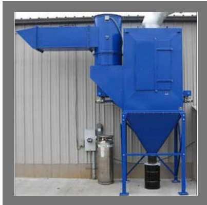
Dust Collection System
