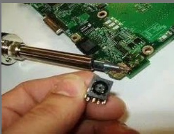
DC Power Jack Repair
