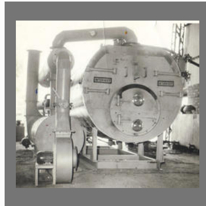
Solid Fuel Fired-wet Back Boiler With Waste Heat Recoveries-2000 Kg Per Hour
