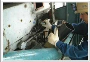
Phased Array Ultrasonic Inspection
