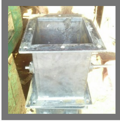
Ms Boiler Dumper
