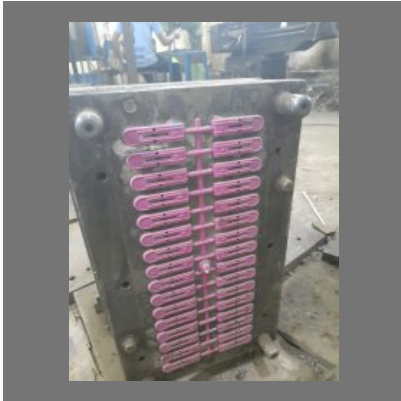
Plastic Cloth Pin Mould
