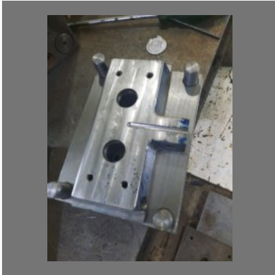
Bottle Cap Mould
