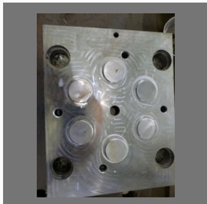
Bottle Cap Mould
