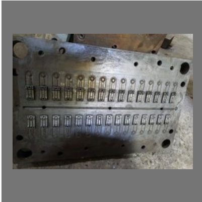
Plastic Clip Mould
