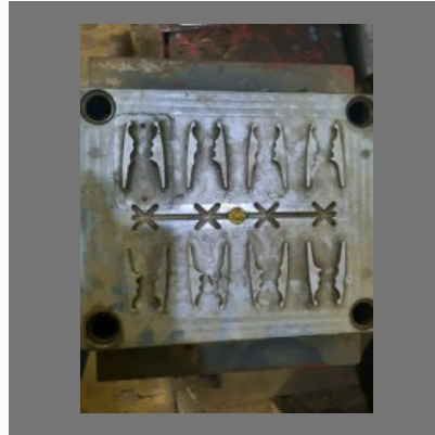
Cloth Pin Mould
