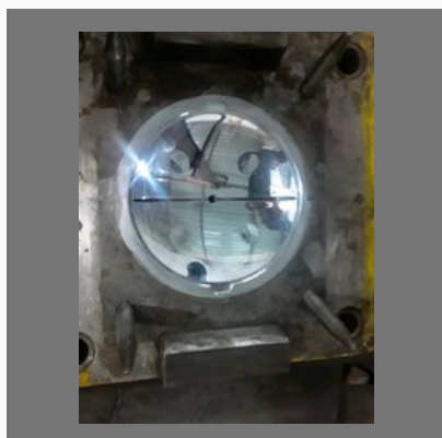
Mixer Jar Cap Mould
