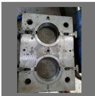
Mixer Jar Bottom Mould
