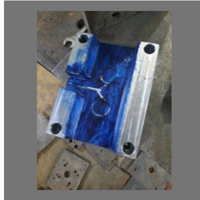
Plastic Cap Mould
