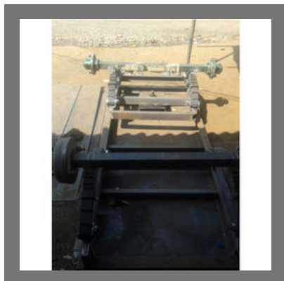
2 Wheel Diesel Generator Trolley
