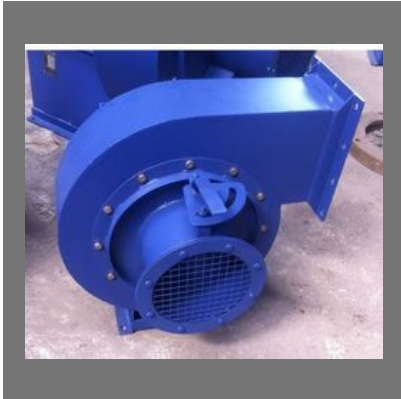
Industrial Centrifugal Blower
