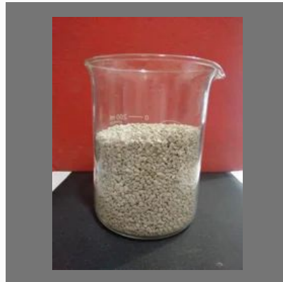
Refractory Boilers Bed Materials
