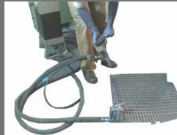
Wire Mesh Repair Welder
