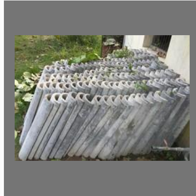
RCC Half Round Pipes
