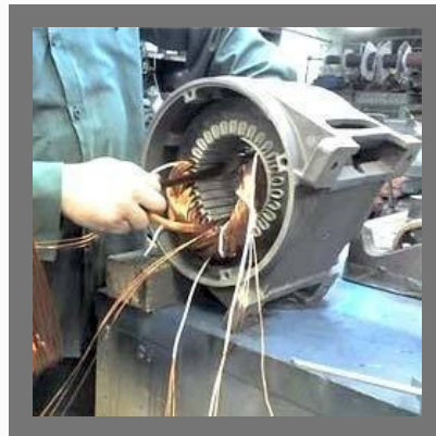
AC Motor Rewinding
