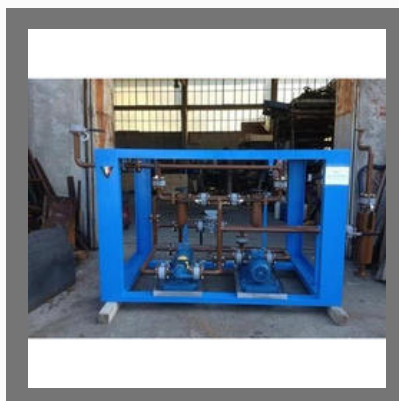
Furnace Oil Pump Unit
