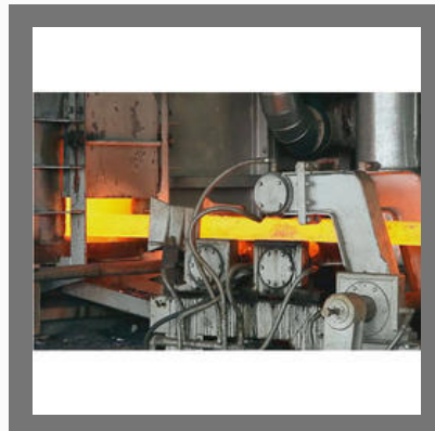
Descaler Steel Hot Rolling Mills
