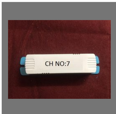
Electronic Ballast Box Choke Box No 7
