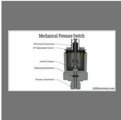
Air Compressor Pressure Switches
