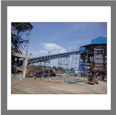
Thermal Power Plant Belt Conveyor
