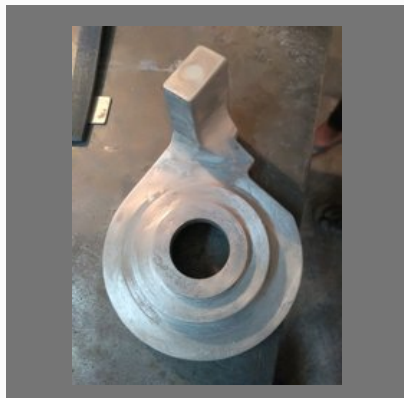
Aluminium Pattern Gearbox Cover
