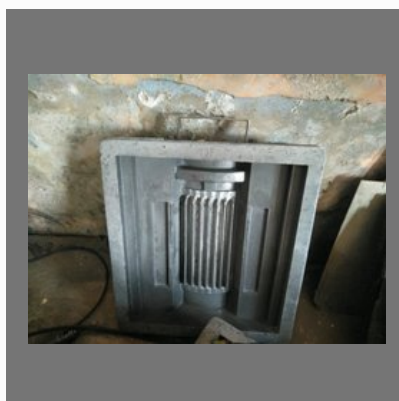
Aluminium Pattern Motor Body
