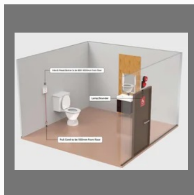
Disabled Toilet Alarm System
