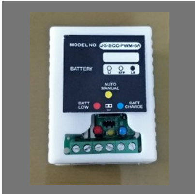
Solar Charge Controller
