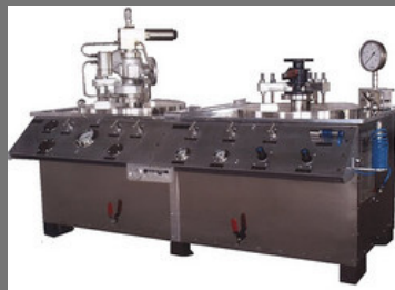
Safety Valve Test Bench
