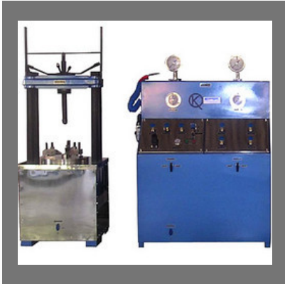
Control Valve Test Bench
