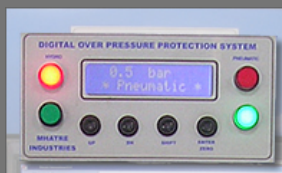
Digital Over Pressure Protection System
