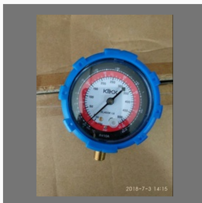
Compound Pressure Gauge
