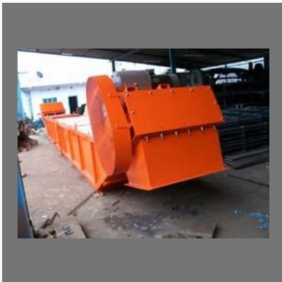
Wet Scraper Conveyor
