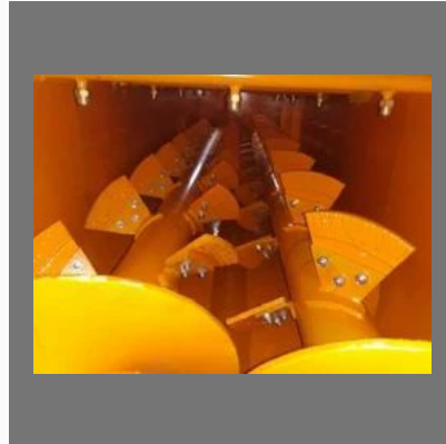
Pug Mill And Dust Conditioner
