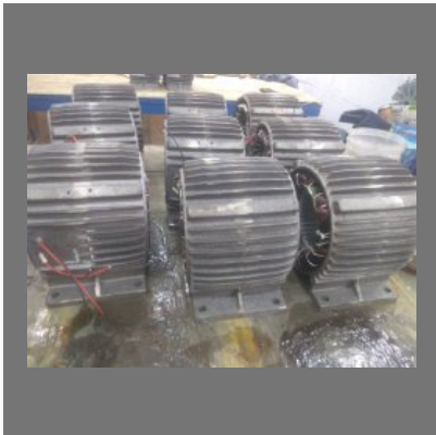
Bore Well Motor
