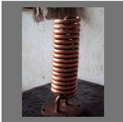
Cooling Coil Heat Exchanger
