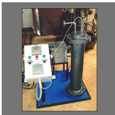
Transformer Oil Heater Heat Exchanger
