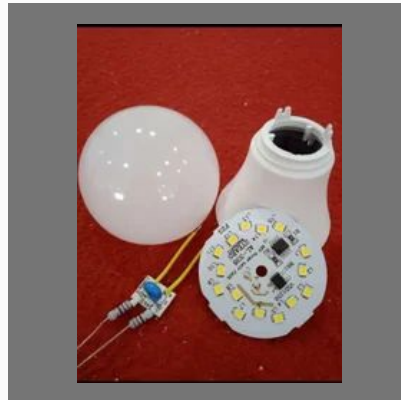
9w Gamma Dob 4kv 440v operating 1mm thickness 46mm
