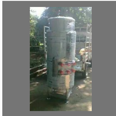
Electrical Steam Boiler
