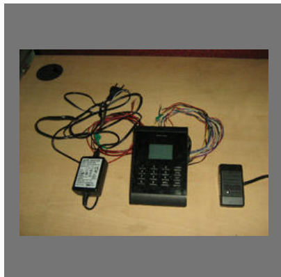
RFID Based Access Control System
