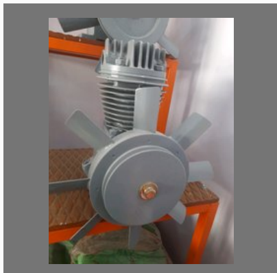
Single Stage Air Compressor
