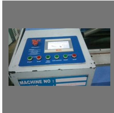
FA225 China Carding Machine PLC Conversion
