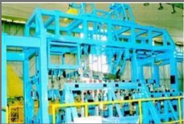
Front Fuselage Assembly Jigs
