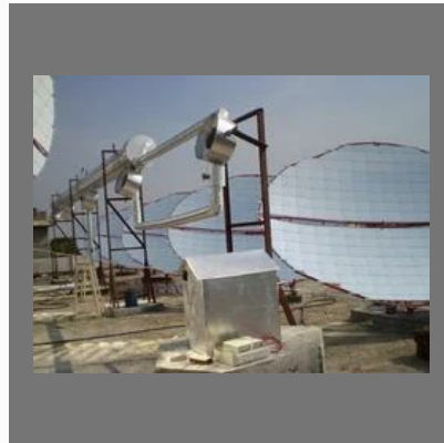
Solar Community Cooking Systems
