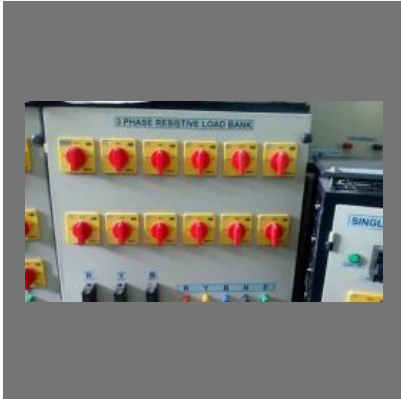
Three Phase Resistive Load
