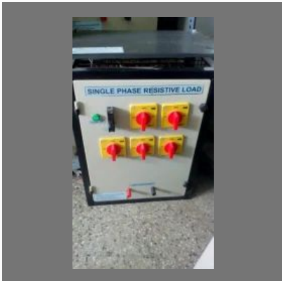
Single Phase Resistive Load
