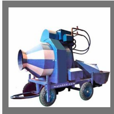
Mobile Batching Plant
