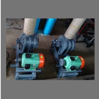
Roots Blower System
