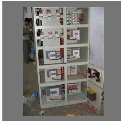
LT Distribution Panels
