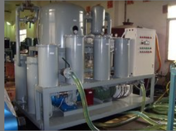
Transformer Oil Filtration Services
