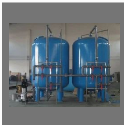
Activated Carbon Filter
